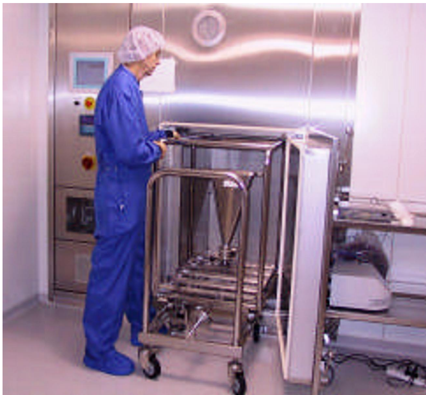
Figure 2: Dry heat steriliser with the door open. Equipment used may be sterilised by dry heat. Product containers will be sterilised by dry heat. In large scale production sterilisation tunnels attached to the washing machine are often used.
