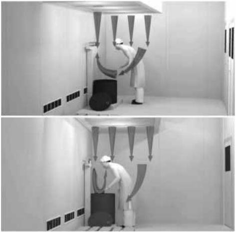
Figure 16 Operator subject to powder inhalation due to worktop obstruction
