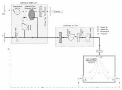
7.5.2 The figure illustrates the chemical drier handling part of the fresh air/return air mixture on a bypass flow. The location of the chemical drier should be considered in the design phase. The practice of locating the complete chemical drier unit in the production cubicle is not recommended as this could be a source of contamination or cross-contamination. Examples of appropriate locations for the drying wheel could include:
