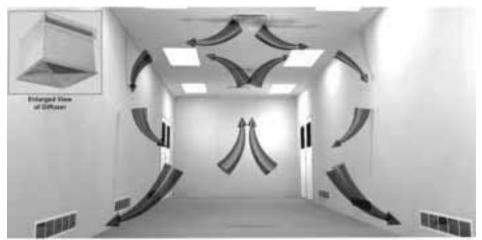
Figure 10 Perforated plate diffuser
