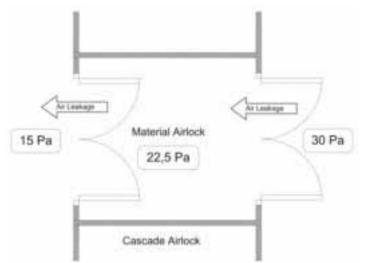
Figure 20 **Example of sink airlock**
