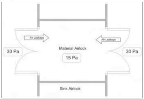
Figure 21 **Example of bubble airlock**
