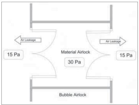
• bubble airlock: higher pressure inside the airlock and lower pressure on both outer sides.
