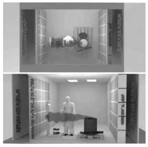
4.3.8 The manufacturer should select either vertical or horizontal unidirectional flow (Figure 17) and an appropriate airflow pattern to provide the best protection for the particular application.
