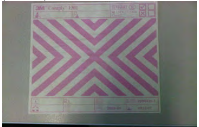
Figure 2. Test sheet showing PASS condition (Pink colour)
