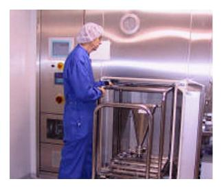
Dry heat steriliser with the door open. Equipment used may be sterilised by dry heat. Product containers will be sterilised by dry heat. In large scale production sterilisation tunnels attached to the washing machine are often used.
